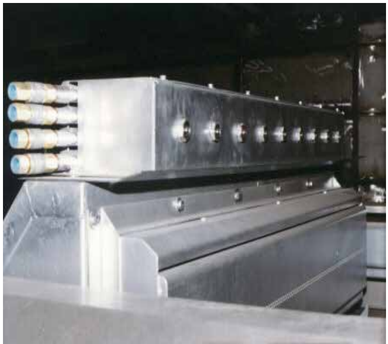
Figure 16 Typical Water Mist Cooling System
